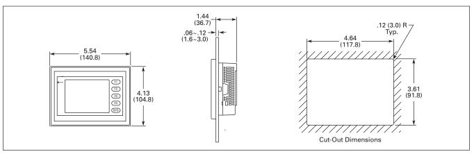
Figure 8. HMI04\_\_ — Approximate Dimensions in Inches (mm)
